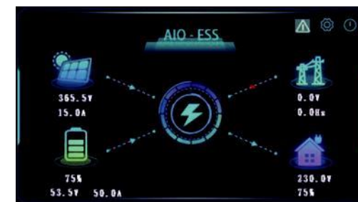
▲ Batteries and solar power supply the load .
