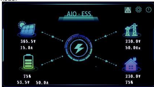
▲ AC Input and solar charging.
